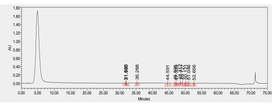
Figure (6): HPLC chromatogram of non-ribosomal lipopeptides in the supernatant of QSLA16. Surfactin determined between 5-35 minutes while fengycin appeared between 35-55 minutes.
